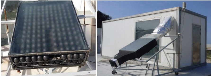
Fig. 1. Double bed solar air collector with latent thermal storage (SAC-2 beds).
