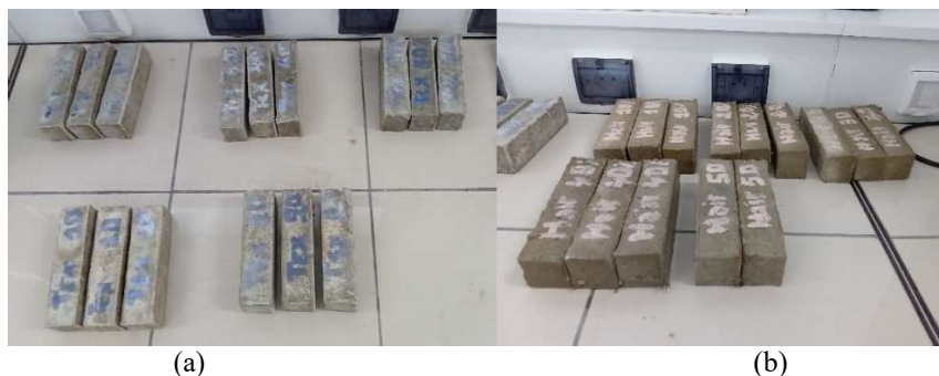
Fig. 1: (a) Textile reinforced mortars, (b) Hair-reinforced mortars after 28 days of curing.
